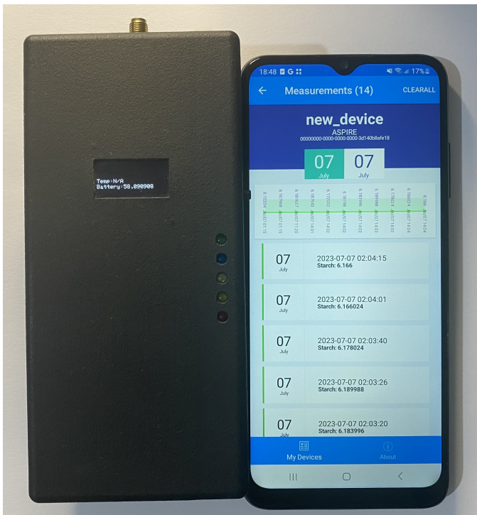
Fig. 3. Starch measurement unit and Android smartphone App. The starch measurement unit transmits data to the smartphone via Bluetooth low-energy (BLE).
