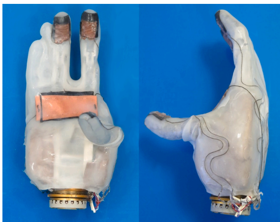
Fig. 3. Silicone glove on the SNAVE hand. Sensors are on the digit tips and on the palm.
