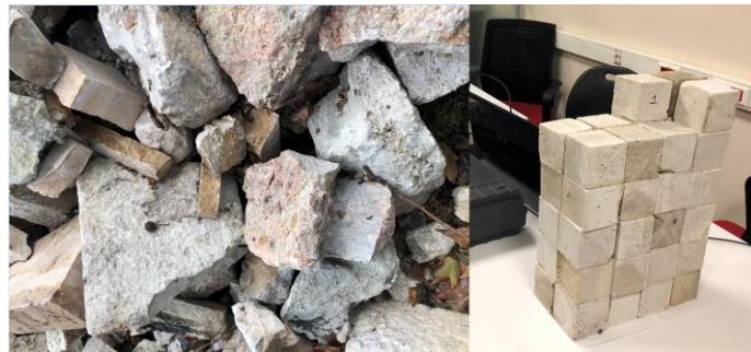
Figure 5. The debris removed from the minaret M3 and the created cubic specimens
