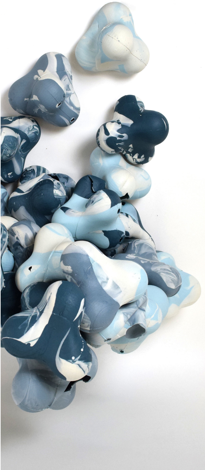
9 Photograph of an aggregation of robotically-assisted rotational cast components, fused to one another during the firing process
