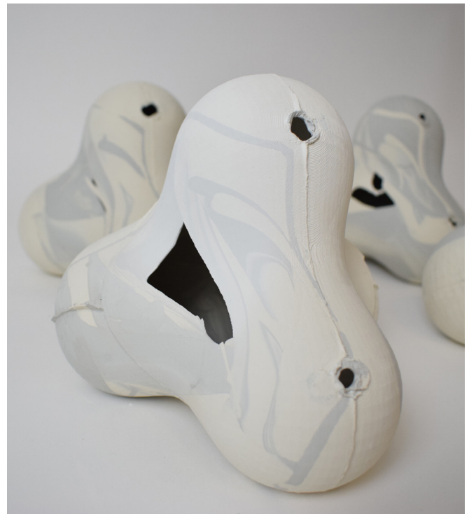
10 A series of robotically-assisted rotational cast components with varying degrees of aperture, as a result of an incomplete coat of the plaster surface
