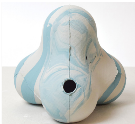
3 Composite image describing the face classification of plaster molds when rotating them by hand alongside two separate casts which produced the same marbling patterns using the same rotational motion while casting. Both of these casts introduce one mason stain of slip into the plaster mold, moving such that sides 0, 1, 2, and 3 faced downward, and repeating with the second color. When side 5 is faced downward after 400 ml of slip is introduced and swirled in that rotation, the pictured effect is achieved.
