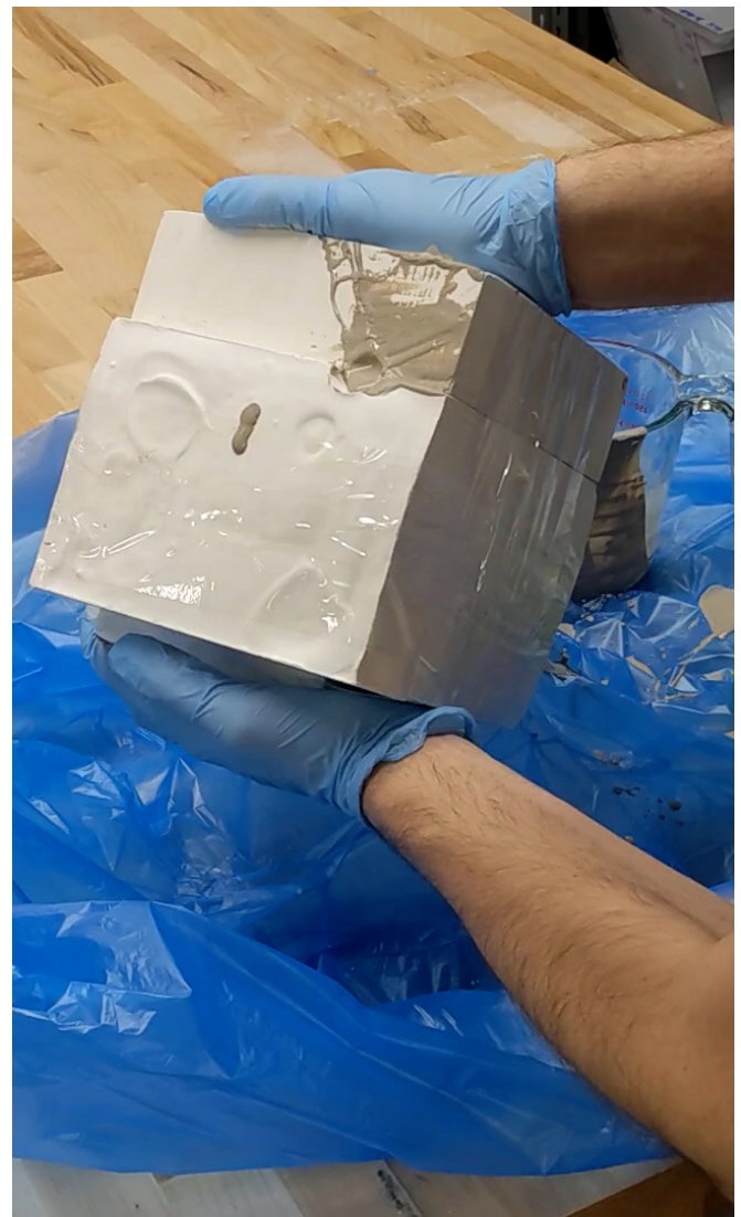
1B A manual test of the robotically-assisted rotational casting process: two colors of liquid slip were poured into a plaster mold and rotated intermittently in order to bring about a controlled marbling effect in the slip cast artifact
