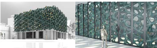
18 (Top) Images of assembled bisque-fired prototype. (Bottom) Renderings of proposed façade.
