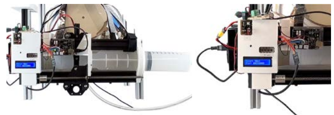
6 Mold holder fabricated attached to the robot.
