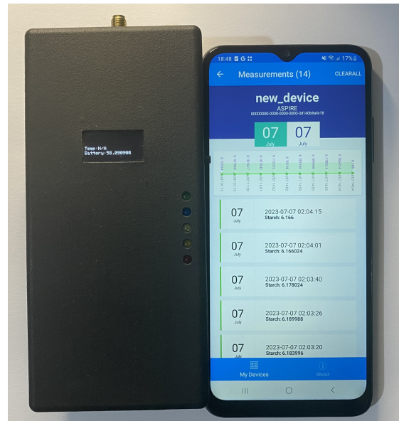
Fig. 6. Version 3 starch measuring instrument together with smartphone App
