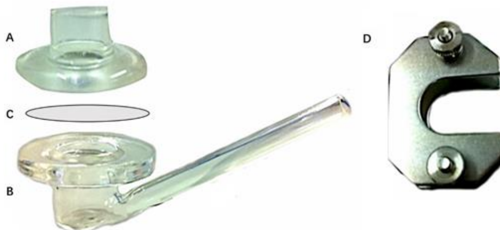
Figure 4.3 Image of the Franz diffusion cells used in following assays. A is the donor chamber; B is the receptor chamber; C is the membrane which would be mounted between the donor chamber and the receptor chamber during permeation; D is the clamp used to fix the diffusion cells.
