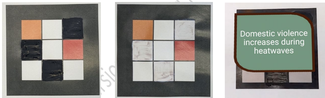
Fig. 8. Thermochromic AR markers shown in a cool state (left), a hot state (center), and overlaid with digitally linked content in AR (right).
