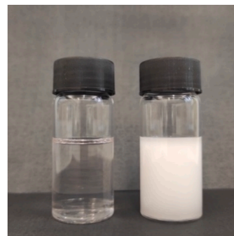
Fig. 6. Photographs of P1 in aqueous solution below (left) and above (right) the LCST.
