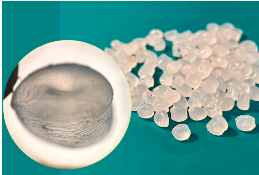
Fig. 2. Image of the plastic nurdles from the Toconao's spill collected at Mexilloeira beach (Ria de Arousa). Collected pellets were white and had an irregular shape. Microscopy photography (close-up on the left) taken with an Olympus CH30 Microscope at 40 \times magnification.
