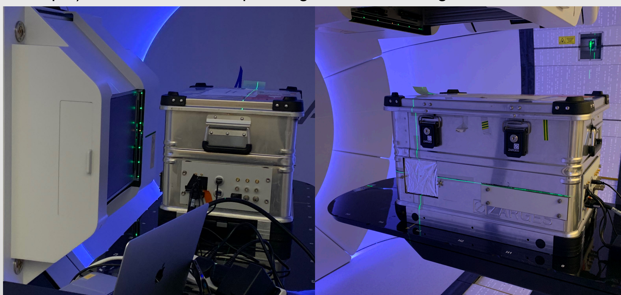
Fig 3. Set-up at UCLH PBT facility. Left: beam nozzle adjacent to the detector housing, containing the scintillator stack and readout electronics. Right: mylar foil beam entrance window and laser-guided alignment system. The first scintillator sheet is placed approximately at the beam iso-centre and an additional window located behind the stack.
