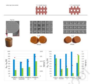
Figure 2: Upper Section: Fabrication of Fe-containing supported monolithic catalysts using the micro-extrusionbased direct-write 3D technique. Lower Section: Comparative assessment of the performance between 3D printed monoliths and their packed bed counterparts in the continuous flow reactor and batch reactor for the oxidation of benzyl alcohol [23]
