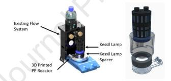
Figure 4: Proposed continuous flow photochemistry system designed to work seamlessly with existing Kessil lamps (depicted on the left). A detailed view (shown on the right) provides an illustration of the suggested lamp setup positioned above the 3D-printed reactor [57].
