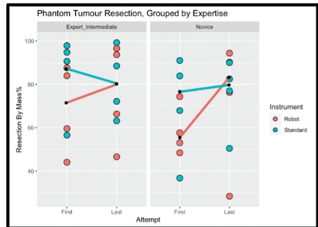
Fig. 3 Graph displaying the extent of phantom tumor resection achieved with the standard instrument versus the robot. Grouped by level of experience. The black circles signify median values for the respective instruments.
