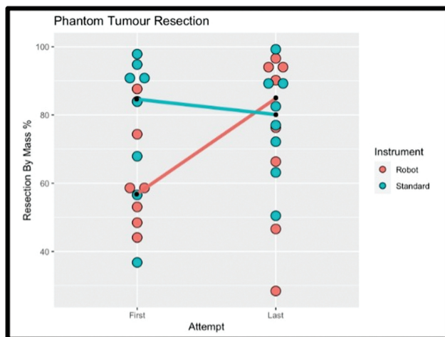
Fig. 2 Graph displaying the extent of phantom tumor resection achieved with the standard endoscopic instrument versus the handheld robot. The black circles signify median values for the respective instruments.
