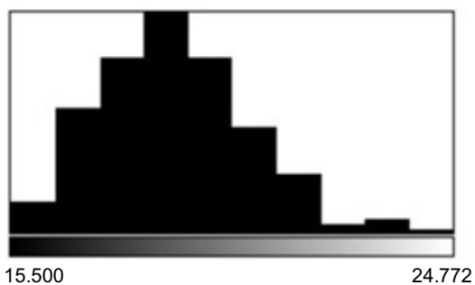
Fig. 1. TEM images of AuNSs at the following magnification: 10.000X (A) and 30.000X (B) and (C) histogram analysis of particle size distribution. Count: 200; mean 18.908; SD: 1.581; bins: 10; min: 15.500; max: 24.772; mode: 18.282 (48); bin width: 0.927.
