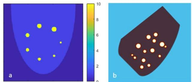
Figure 3. Phantom with two layers of 7 spherical inserts; a) transaxial (x-z) plane, b) maximum-intensity projection at an oblique angle, showing all spheres.
