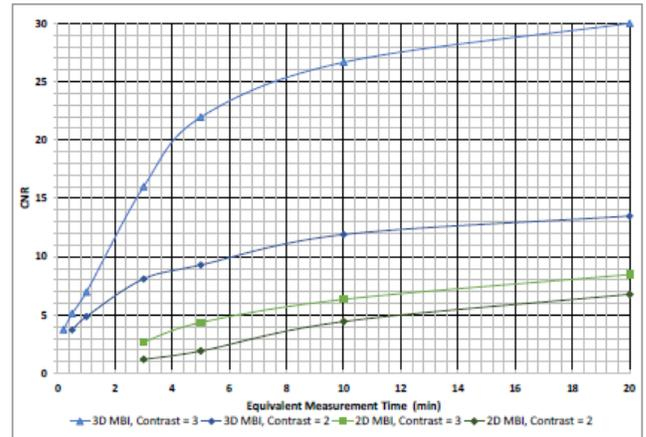
Figure 8. CNR values for different tumour-background ratios (contrast = 2 and 3) as the function of measurement time. Blue lines represent the values measured with the multi-pinhole 3D MBI prototype, while green lines show simulated 2D parallel-hole data.
