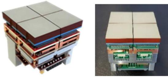
Figure 1. Detector module used in the proof-of-principle prototype (left) and the new feasibility prototype (right).
