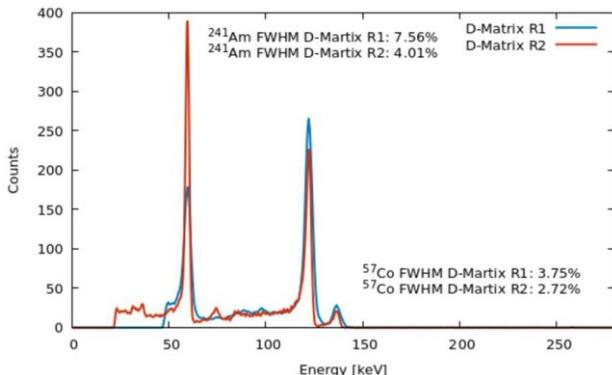
Figure 6. Comparison between the raw  $^{57}\text{Co}$  spectra measured with previous D-Matrix R1 (blue line) and new R2 (red line) system.
