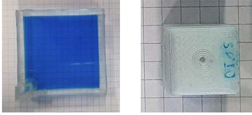
Figure 4. Homogeneous box phantom (left) with 30 x 30 x 20 mm cavity and spherical phantom (right) with a cavity of 6 mm in diameter.
