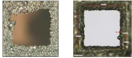
Figure 2. 3D printed tungsten collimator hole picture from the first proof-of-principle prototype (left) and new feasibility prototype (right).
