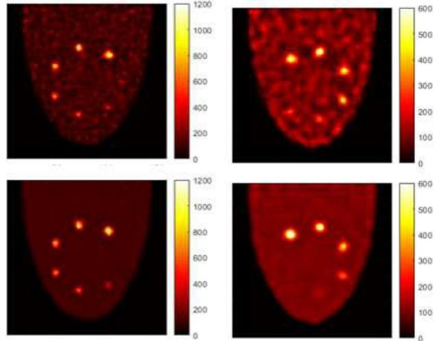
Figure 7. Reconstructed images from the simulation study from close to the detector (left) and middle (right) planes without (top) and with (bottom) NLM noise filtering.
