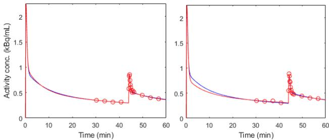
Fig. 3. Simulated AIFs, including true curves (blue), sampled values (circles) and fitted curves (red) for 20% 2<sup>nd</sup> inj. protocol, with good (left) and less good (right) agreement.
