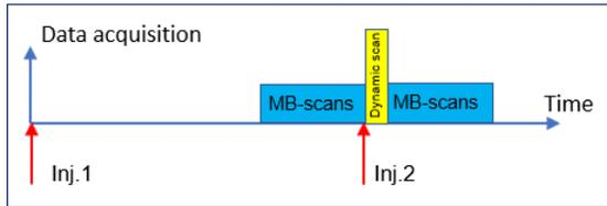
Fig. 1. Dual-injection protocol with a series of multi-bed (MB) scans, starting some time after the 1<sup>st</sup> injection, a short dynamic acquisition directly after the 2<sup>nd</sup> injection, and then another series of MB-scans.
