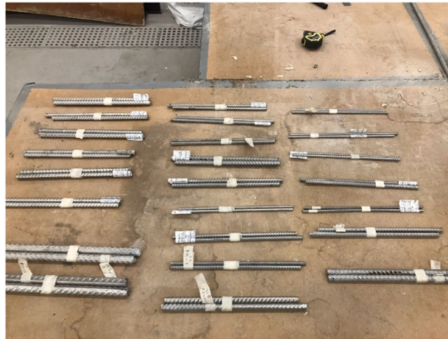
Fig. 2. Stainless steel reinforcement bars before tensile testing.
