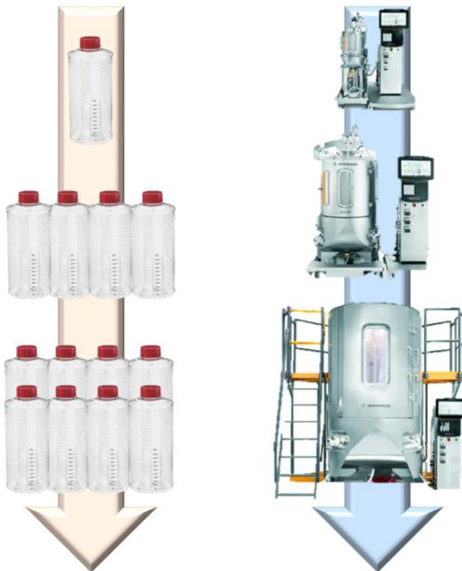
Figure 1.6 Schematic highlighting the methods of increasing culture volume for AAV production. On the left, roller bottles, an example of an adherent culture technology, whereby scaling out is required to permit an increase in culture volume. On the right, a single use bioreactor as an example of a suspension culture technology; in this case, scale up is possible. Note: bioreactor images sourced from Sartorius, roller bottle images sourced from Sigma Aldrich.
