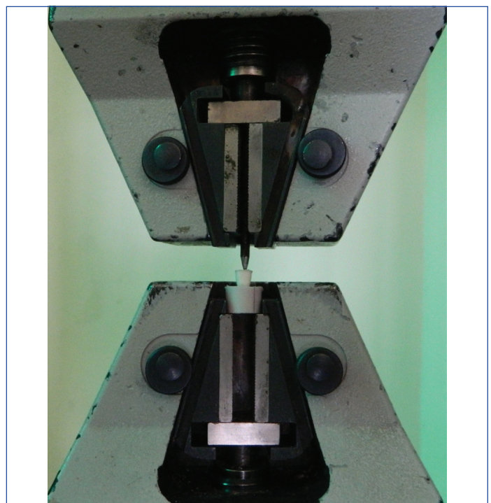
[Table/Fig-3]: Mounted tooth was placed on the universal testing machine for mechanical testing.
