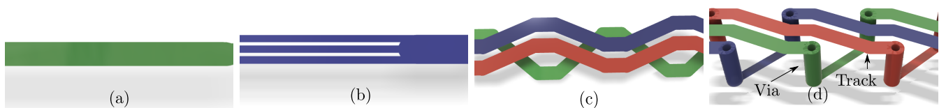
Figure 1. Conductor structures studied in this paper. (a) Solid track structure, (b) multitrack structure, (c) in-layer twisted structure (the red and blue tracks are located on the top layer of the PCB, while the green track is located on the bottom layer. This system incorporates an in-layer horizontal movement between the different subtracks within each turn), and (d) Litzing structure (in addition to the horizontal movement within the layers, the Litz structure also incorporates vertical movement between layers using vias).
