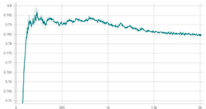
Fig. 5. Y-axis: Learnt threshold in the experiment of Task05 Prostate. X-axis: training iterations. The mean of the prior is 0.9 and the std of the prior is 0.1. The learnt threshold converged around 0.785 after 2000 iterations.
