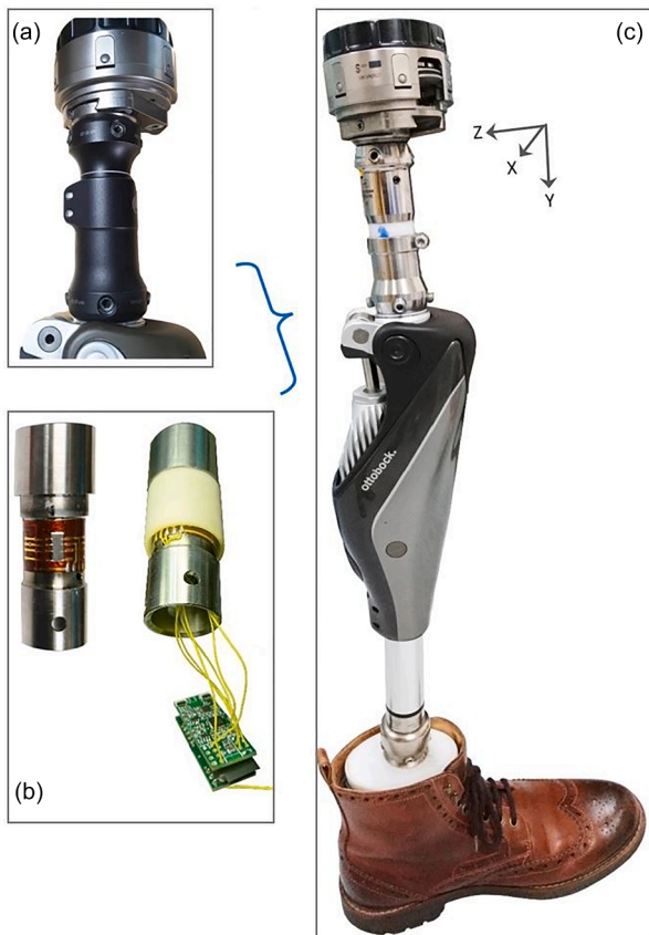
Fig. 1. (a): Prosthetic tubing before load cell replacement. (b) Load cell with one flat and gold wires on a flexible circuit pad before and then after fitting the protective plastic collar and wired to electronics. (c) Final assembly with load cell replacing prosthetic tubing.
