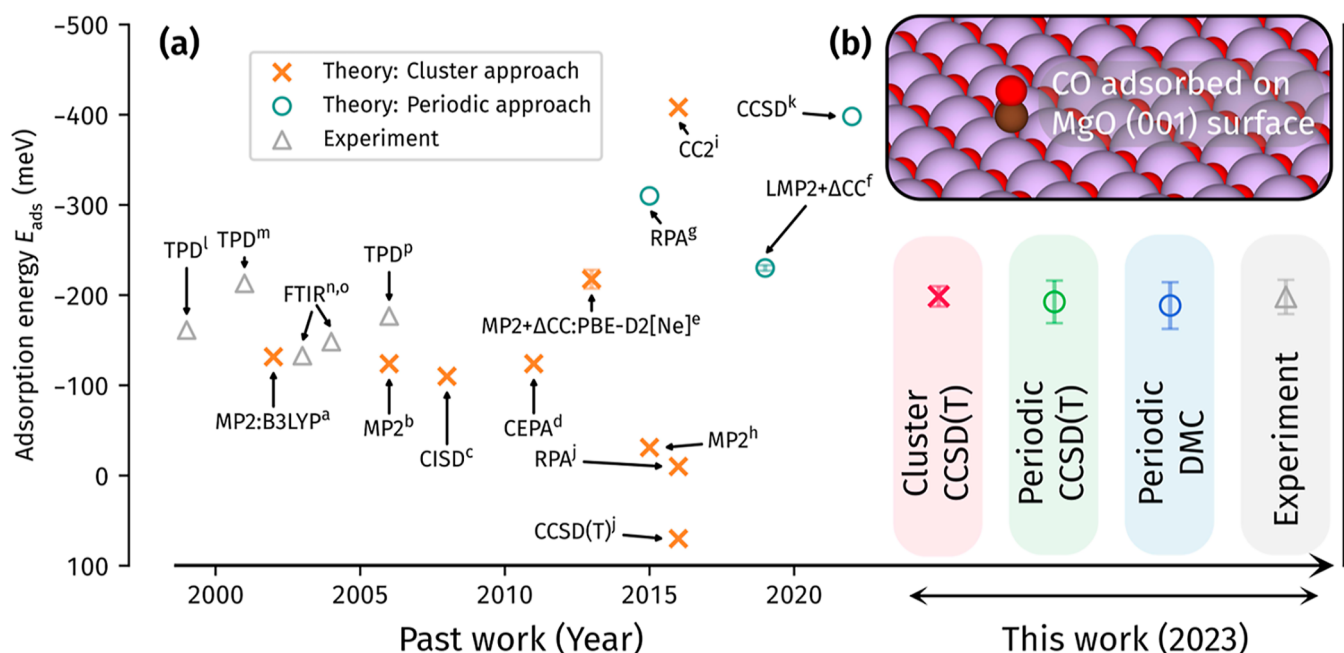
Figure 1. (a) Adsorption energy E_{\text{ads}} of CO on MgO from previous experimental and theoretical investigations. For the past theory work, we focus on many-body wave function studies employing either a cluster or periodic approach. The past experimental work involves either the Fourier transform infrared (FTIR) or the TPD technique, which we discuss in Section S9 of the Supporting Information . The CO on MgO system is visualized in the top panel of (b), and in its bottom panel, we give accurate estimates to E_{\text{ads}} from this work utilizing CCSD(T) with a cluster approach, CCSD(T) with a periodic approach, and DMC with a periodic approach. A best estimate of the experimental value has also been made by reanalyzing the previous experimental work with an improved pre-exponential factor (discussed in the text). Error bars have been determined for all estimates made from this work. References for past simulation work are as follows: (a) Ugliengo and Damin, 20 (b) Herschend et al., 21 (c) Qin et al., 22 (d) Staemmler, 23 (e) Boese and Sauer, 24 (f) Alessio et al., 25 (g) Bajdich et al., 26 (h) Li et al., 27 (i) Heuser and Höfener, 28 (j) Mazheika and Levchenko, 29 (k) Mitra et al., 30 References for past experiments are as follows: (l) Wichtendahl et al., 31 (m) Dohnálek et al., 32 (n) Spoto et al., 33 (o) Spoto et al., 34 (p) Sterrer et al. 35
