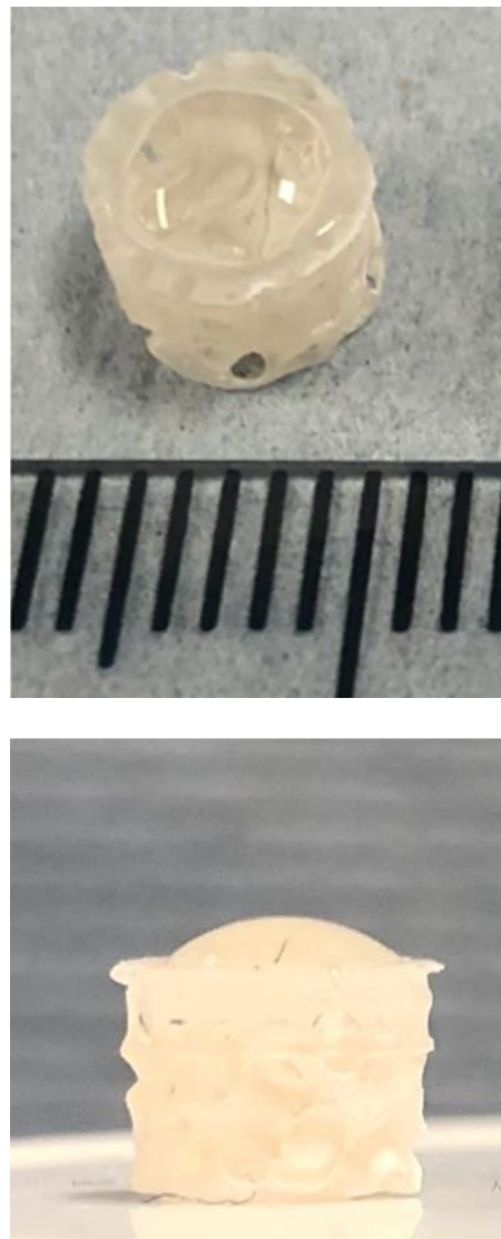
Figure 4. 3. The physical appearance of the GelMA/CSMA-2 Bilayer scaffold.
