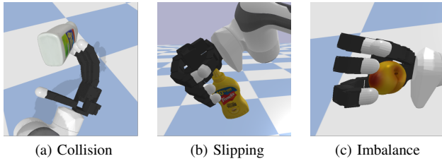
Fig. 12. Representative examples of failure modes: (a) collision before catching, (b) slipping from the grasp or (c) imbalanced contact points.
