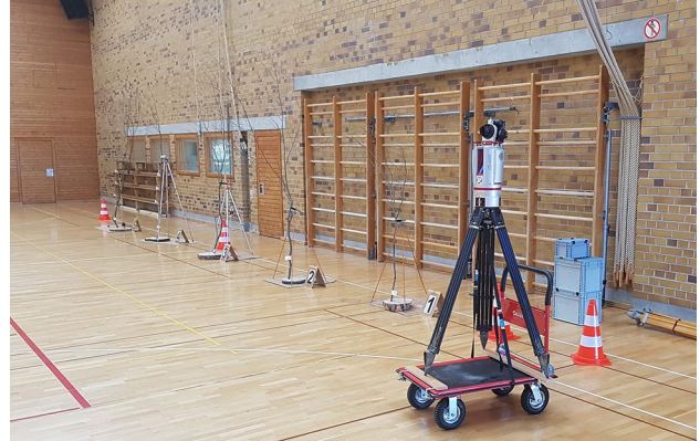
Fig. 7 Scanning setup of one set of five branches. The branches were stabilised using platforms and tripods. The scanner was mounted to a trolley to facilitate scanning
