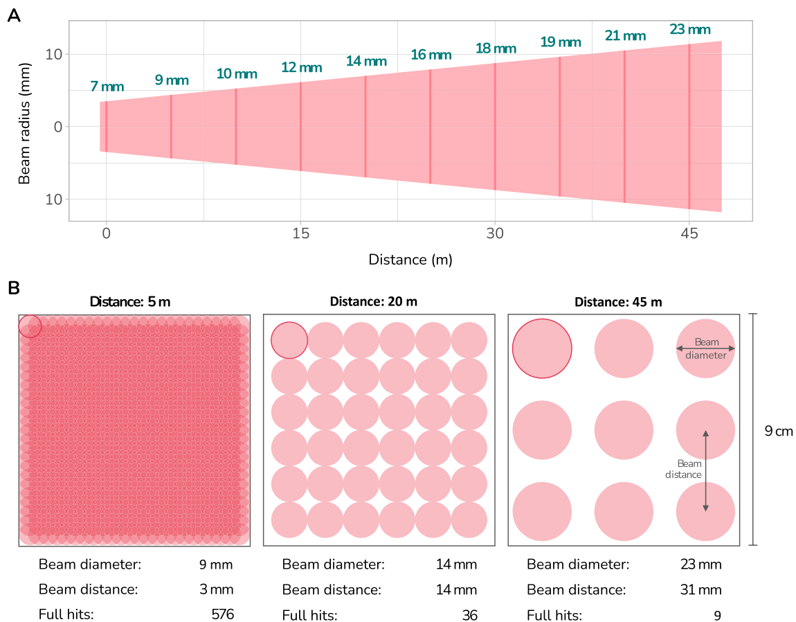
Fig. 2 a Laser beam radius and diameter (mm) of the RIEGL VZ-400i depending on the distance to the scanner. b Laser beam diameter (mm) and distance between the centres of the laser beams (mm) and number of full hits on a target area of 9 cm × 9 cm with increasing
