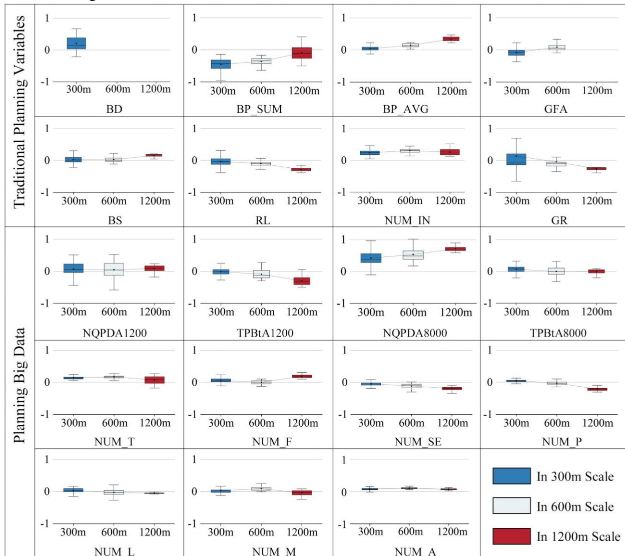
Fig. 9. Variations in the impact of planning variables on traffic noise level with scale
