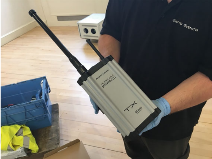
Fig. 7 Euan Kerr from Zisys Events holding the Xirium Pro transmitter prior to installation on the roof of Modern One (Photo: Brian Castriota)
