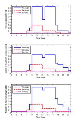
Figure 4. ASHRAE 90.1 schedules for occupancy (top), lights (middle), and plug loads (bottom) used in modeling scenario 1a.
