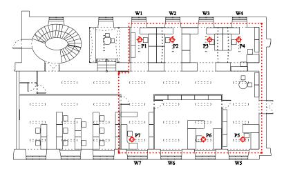
Figure 20. Schematic illustration of the office area, observed occupants (P1-P7) and operable windows (W1-W7).
