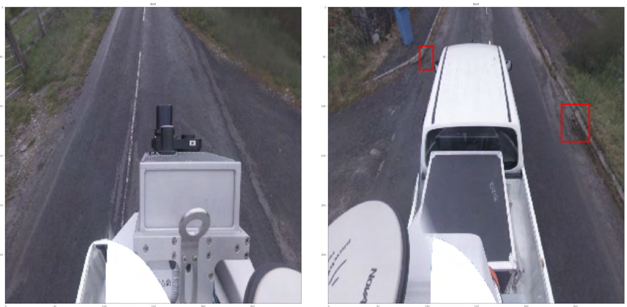
Figure 9: Example of gnomonic projection of spherical image in Figure 7 with P = (0.75, 0) (left) and P = (0.75, 0.5) (right).
