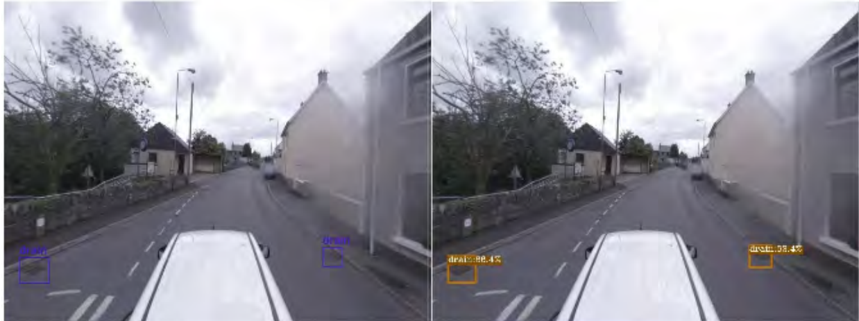
Figure 28: Example of Drainage Detection using the YOLO model. The left image includes ground truth annotations in purple and the right image is output from the detection model with the detected drainage locations.
