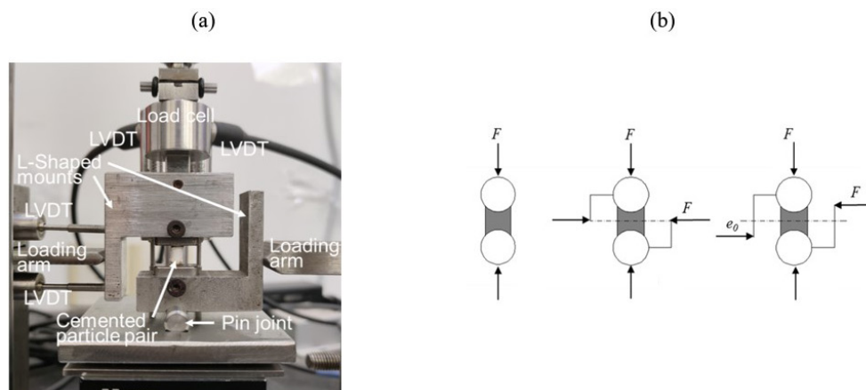
Figure 3. Inter-particle loading apparatus for cemented particles: (a) photo; (b) schematic (modified from Wang et al., 2019).
