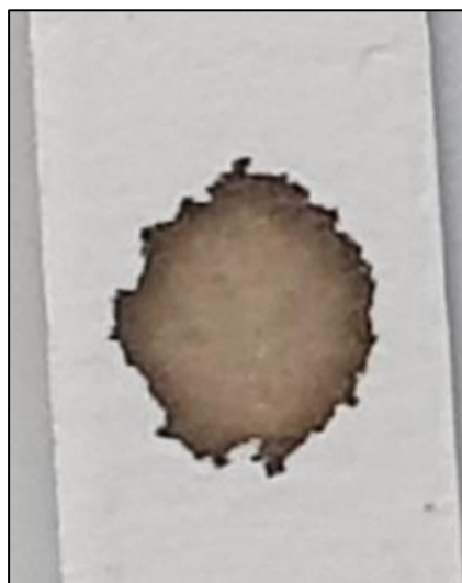
Figure 1 Coffee ring formation of MNPs@citrate on a nitrocellulose membrane.
