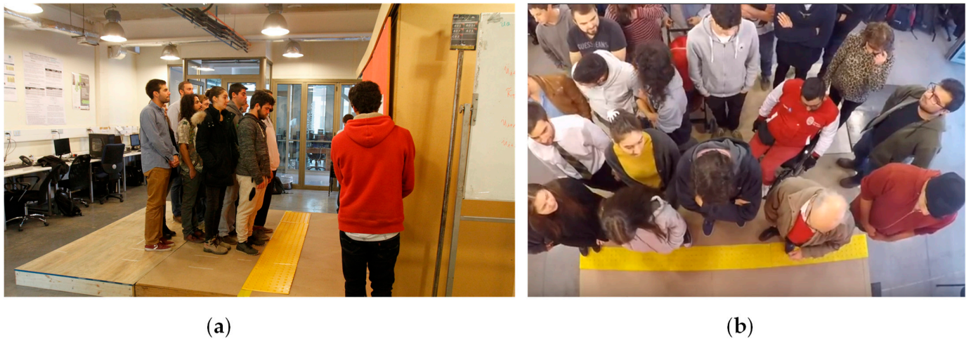
Figure 2. Laboratory experiments to represent the boarding and alighting: (a) lateral view of the platform when passengers are waiting to board the train and (b) top view of the platform when passengers are waiting to board the train.
