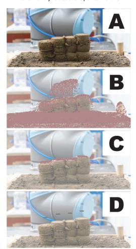
Figure 4 a) unequal layer height, b) scanned point cloud, c) isolated top layer, d) offset planes for next layer. Table 1 Deviation of place position with scanner
