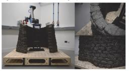
Figure 1 Impact Printing of Cob
