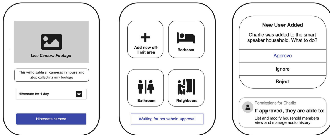
Fig. 4. Consent and permission smart homes features designed by participants using heuristics: (a) hibernate feature for smart cameras that temporarily stops cameras from collecting footage; (b) off-limits feature for smart cameras that restricts areas in the home from being recorded; and (c) permissions feature for smart speakers that requires household approval to add new members.
