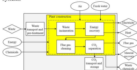
**Figure 3:** Schematic representation of the LCA system boundaries.
