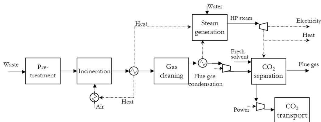
**Figure 1:** Schematic of the steps modelled to simulate the operation of Waste-to-Energy retrofitted with CCS.
