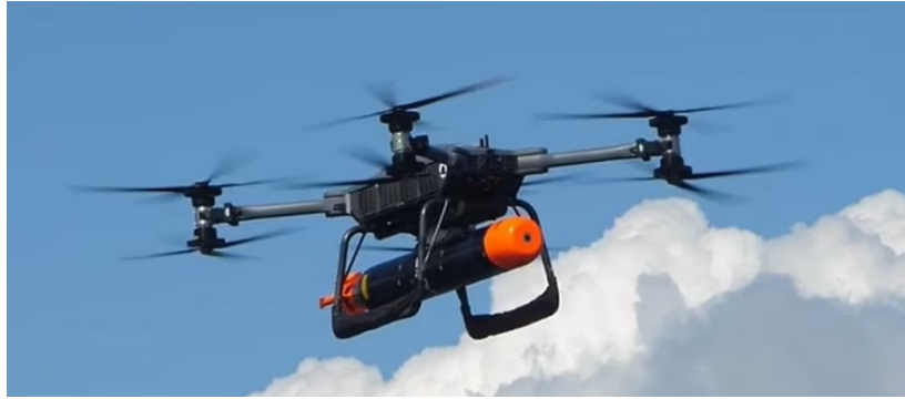
Figure 3 – BAE Systems T-650 Drone carrying a lightweight anti submarine torpedo [BAE SYSTEMS}
