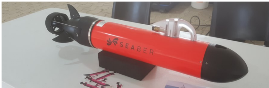
Figure 4 – SEABER Small modular UUV, REPMUS 2023 trials
