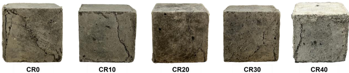
Fig. 9. Typical compressive failure patterns of EGC with various crumb rubber contents at 28 d.
