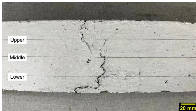
Fig. 4. An example of how to determine the crack number and crack width of EGC.
