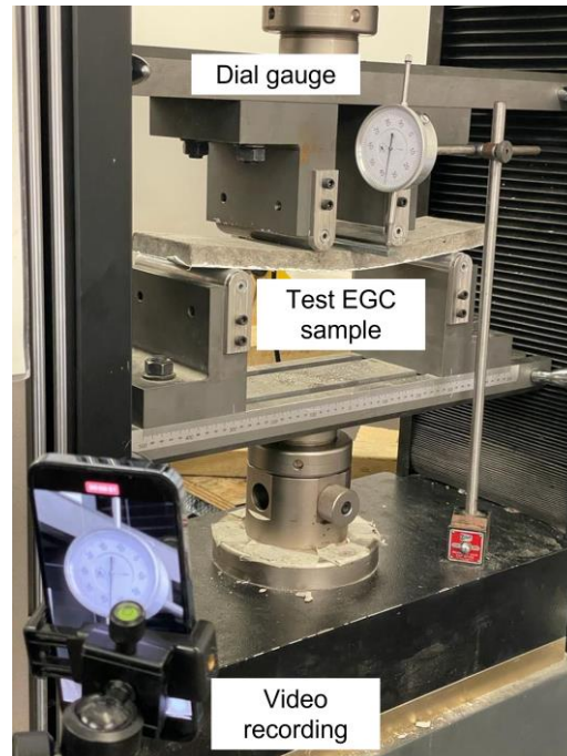
Fig. 3. A photo of four-point bending test setup.
