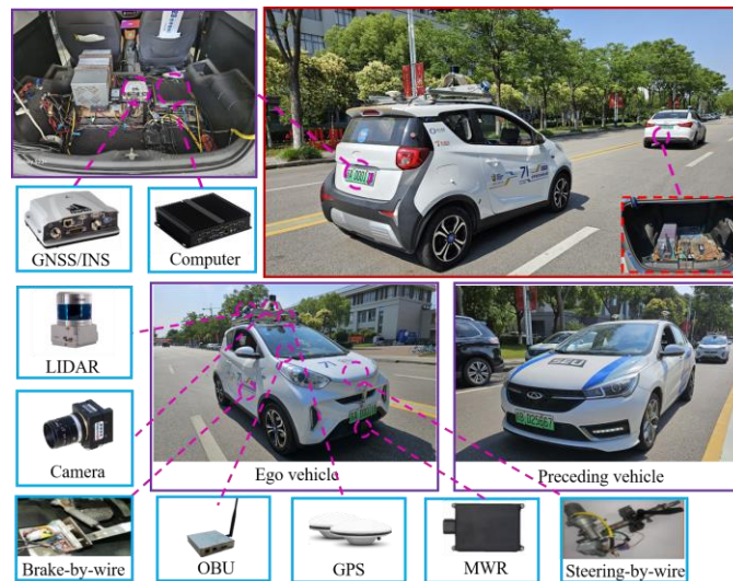
Fig.23. The experimental platform and test road for the connected and automated vehicle.
