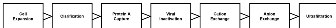
Fig. 1. Flow diagram of the bioprocess stages for mAb manufacture. Eluates were from Protein A capture chromatography, viral inactivation, cation exchange, anion exchange and ultrafiltration.
