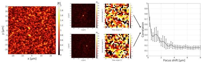
Figure 3. A plane wave propagating through a tissue-like medium is scattered and a speckle pattern is generated. A stepwise sequential algorithm is used to optimise the phase of the incident light to produce an optical focus at an arbitrary location within the imaging plane. The correlations between the phase maps used to optimise a focus at a given location along the x-axis are calculated and plotted.
