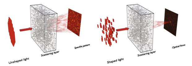
Figure 1. Light incident upon a highly turbid medium is strongly scattered. However, appropriately structured light propagates through the same medium in such a way that the transmitted field constructively interferes within a target region, producing (in this example) an optical focus. Depicted speckle patterns are physically realistic simulation data generated by shaping light through a titanium dioxide (TiO2) medium.
