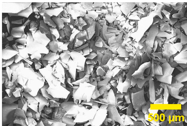
Fig. 9. SEM images of ZnS sheets produced from the dry decomposition of 2b .
