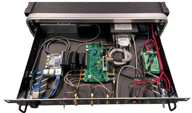
FIGURE 10 Photograph of a single node of the RadSync GNSS Disciplined Oscillator (GNSSDO) based multistatic radar synchronisation system. Raspberry Pi (RPI) single board PC (far left); Custom interface card (centre). Uninterruptible-Power-Supply (UPS) (far right). LNRCLK GPS Disciplined Oscillators (GPSDO) visible in top right and Thunderbolt E GPSDOs (THUN-E) GPSDO visible top left.
