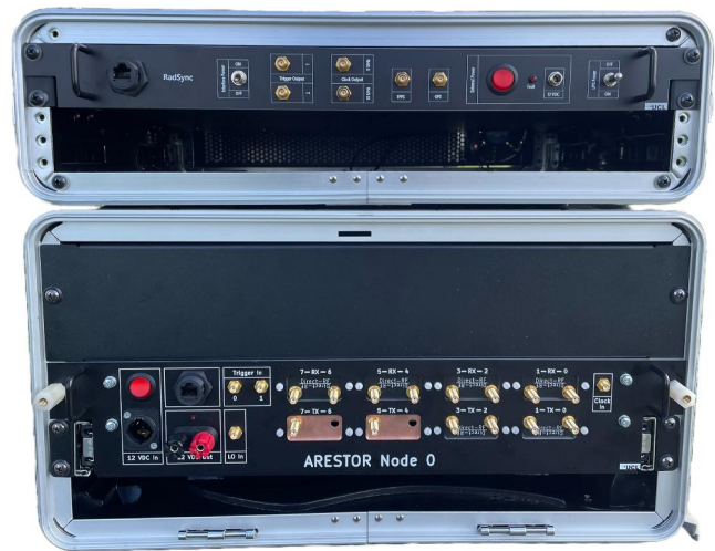
FIGURE 18 Photograph of a single node of the multistatic radar system. ARESTOR multi-functional RF system node in bottom 4U rack. RadSync Global Positioning System (GPS) Disciplined Oscillator Synchronisation System node in 2U rack above.
