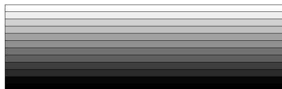
Figure 2. Division of an FG-CNTRC beam into uniform homogenized sub-layers.
