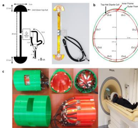
Figure 1. Top-hat dipole reception RF coil. (a) the integrated view. (b) the inner and outer frame design. (c) Separated inner (red) and outer (green) frames showing the coil attached.
