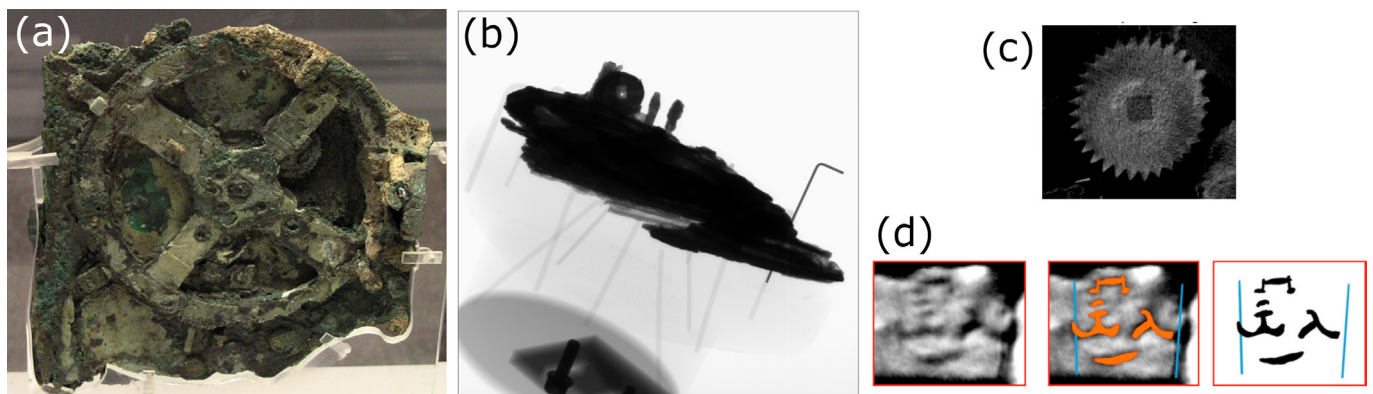
Figure 3. (a) is a photograph of Fragment A, the largest fragment of the Antikythera Mechanism (from en.wikipedia.org/wiki/Antikythera_mechanism, licensed under CC BY 2.5). (b) shows one X-ray CT projection of the Mechanism; (c) shows one reconstructed gearwheel; (d) shows reconstructed text and its interpretation (b, c and d are cropped from Pakzad et al 13 and are licensed under CC BY 4.0 (creativecommons.org/licenses)).
