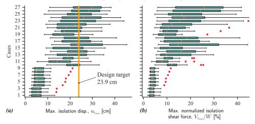
Figure 7. Boxplots for the demand parameters of the X-direction isolation system: a) maximum displacement  $u_{i_{max}}$ , and b) maximum normalized shear force  $V_{i_{max}}/W$ .
