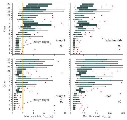
Figure 8. Boxplot for the demand parameters of the superstructure in X-direction: maximum inter-story drift  $\Delta_{max}$  of: (a) first story; (c) third story; and maximum floor accelerations  $\ddot{u}_{max}$  of (b) isolation slab, and (d) celing of third story (roof).
