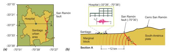
Figure 1. (a) Plan view of the Metropolitan region; and (b) schematic cross-section East-West, including a schematic representation of the San Ramon Fault
