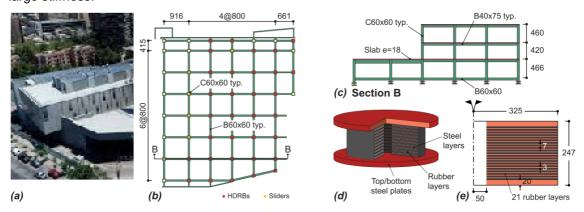
Figure 2. Case-study hospital building: (a) aerial view; (b) plan view of the isolation system; (c) typical elevation of the isolated structure; and (d - e) scheme of the HDRBs.
