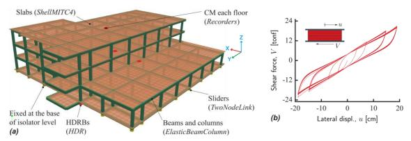
Figure 3. Case-study building: (a) 3D view of the FE model, and (b) shear force-lateral displacement hysteresis of the HDRB model.
