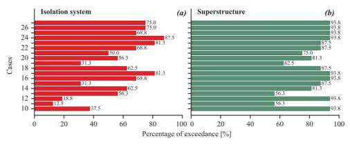
Figure 9. Probability of exceedance of two limit states for the different earthquake scenarios: (a) isolation system, and (b) superstructure.
