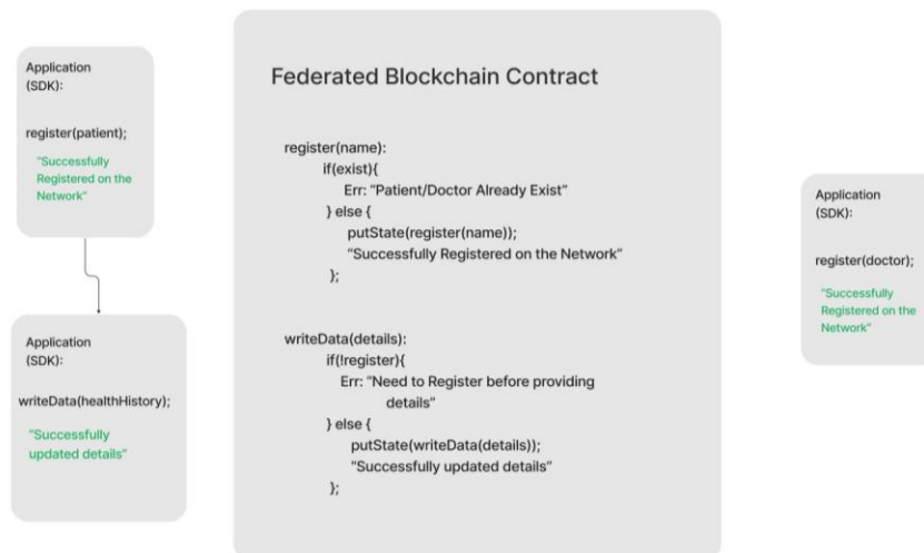
Figure 3. Schematic showing a sample federated blockchain contract for user registration, and writing the basic details.
