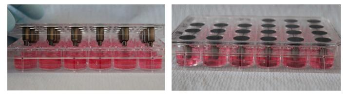
**Figure 3.** Inverted sample attached lids (SAL) serving as a vehicle or carrier to hold the specimens directly hanging over the culture.
