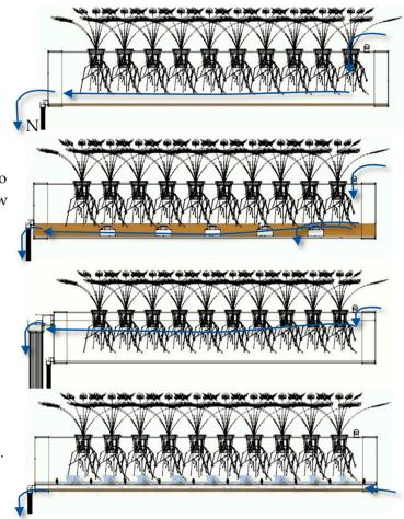
Figure 1. Cross-section drawing of the different hydroponic setups and flow direction of sewage.
