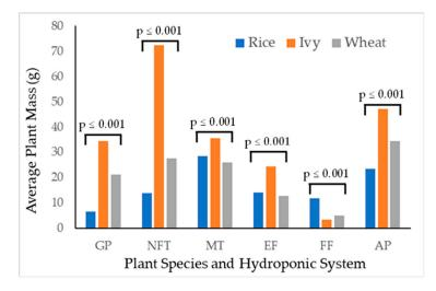
**Figure 2.** Change in mass (g) for all experiments for the rice, ivy and wheat grass. The tomato experiment is not shown as the plant growth failed. Geyser pump (GP), nutrient film technique (NFT), misting (MT), ebb and flow (EF), full flow (FF), aeroponics (AP).
