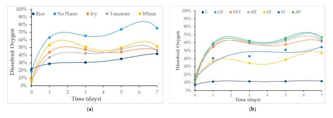
**Figure 5.** (a) Average DO throughout the experiment for all the systems averaged to the experiment run. (b) Average DO throughout the experiment for all the systems. Geyser pump (GP), nutrient film technique (NFT), misting (MT), ebb and flow (EF), full flow (FF), aeroponics (AP), control (C).
