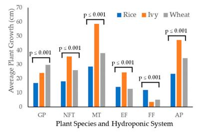
**Figure 3.** Total growth of the plants including root and body parts of the plants. Geyser pump (GP), nutrient film technique (NFT), misting (MT), ebb and flow (EF), full flow (FF), aeroponics (AP).
