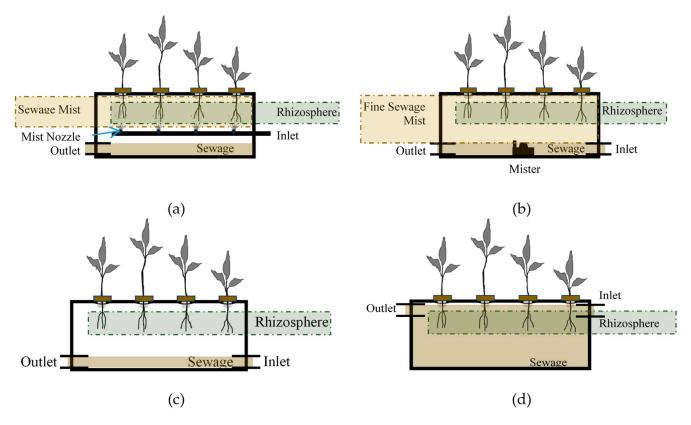
**Figure 6.** Schematics of the AP (**a**) and MT (**b**) systems showing the zone of moisture that encourage the growth of the rhizosphere. NFT (**c**) system showing the stream of sewage above the rhizosphere zone. A schematic of an FF (**d**) system showing that the rhizosphere was smothered in sewage restricting its access to oxygen.
