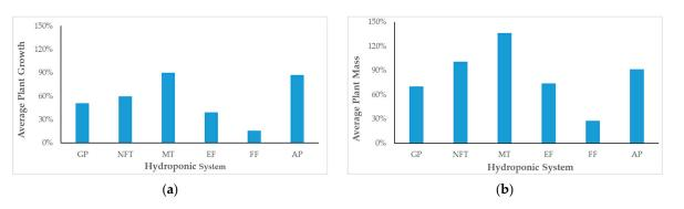
**Figure 4.** Average growth as a measurement of length (**a**) and mass (**b**) as a percentage for each system across all experiments. Geyser pump (GP), nutrient film technique (NFT), misting (MT), ebb and flow (EF), full flow (FF), aeroponics (AP).
